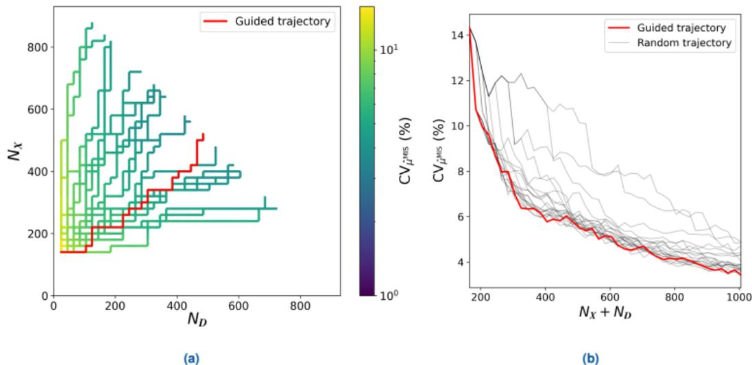
**Figure 3.4:** Comparison between the guided trajectory and random trajectories of enrichment. (a) Trajectory of enrichment guided by sensitivity analysis (in red) alongside 20 random trajectories. (b) Coefficient of variation assessed during data enrichment. *The coefficient of variation related to the guided trajectory (in red) is one of the lowest.*
