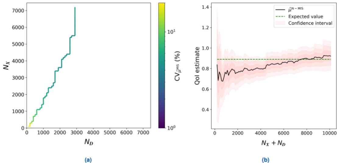
**Figure:** Approach applied to a test case of a firespread of dimension  $q = 10$  with a **sample of experiment** of initial size  $N_D = 25$  and a **sample of simulations** of initial size  $N_X = 140$ . The enrichment step is set to 100. (a) Trajectory of enrichment taken by the algorithm for the cantilever beam toy case. (b) Estimation of the QoI during data enrichment.
