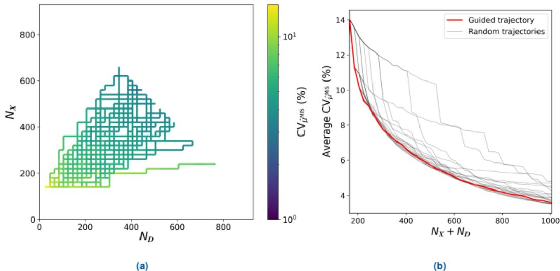
**Figure 3.5:** Repetition of the approach. (a) Trajectory of enrichment guided by sensitivity analysis obtained on 40 repetitions. (b) Average coefficient of variation assessed on 40 repetitions during data enrichment. *The coefficient of variation related to the guided trajectory (in red) is one of the lowest.*
