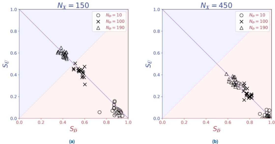
**Figure:** Evolution of Sobol' indices for the cantilever beam toy-case at  $N_D = [10, 100, 190]$  and (a)  $N_X = 150$  (b)  $N_X = 450$ . Estimation of  $r = 20$  indices for each combination.
