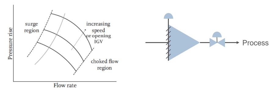
The term "surge" is used to denote an uncontrolled flow process in the compressor. It is defined as the operating point at which the compressor peak head capability and minimum flow limit are reached. At this point, the compressor loses the ability to maintain the peak head and the entire system becomes unstable. This results in conveyed fluids flowing back from the discharge side to the suction side resulting in admissible load reversals on the blading.
