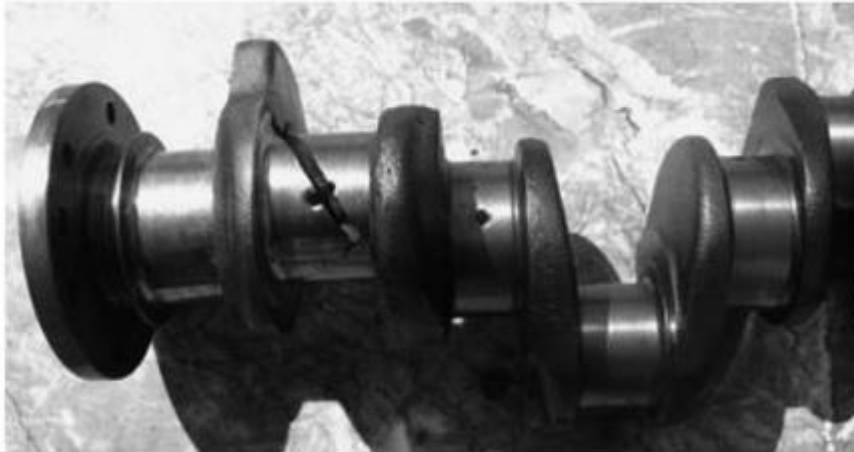
Crack location in a failed crankshaft [1]
