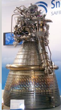
Vulcain 2 Liquid Propulsion System
